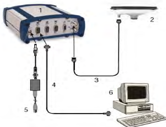
Figure 5.1: The SCINDA GPS setup and installation
