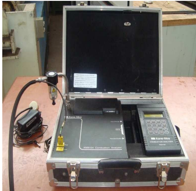
Fig. 5.17: Combustion gas analyser KM9104
