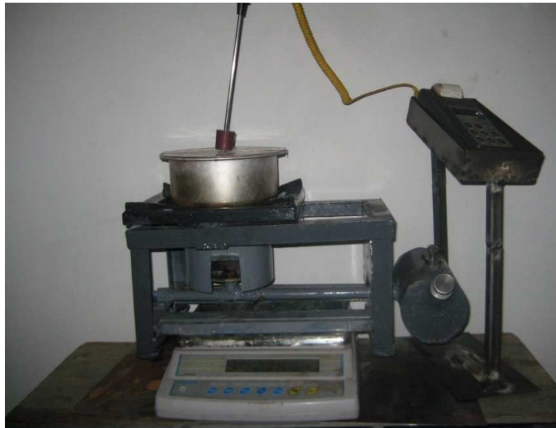
Fig. 4.1: Stove system with temperature measurement set-up and scale
