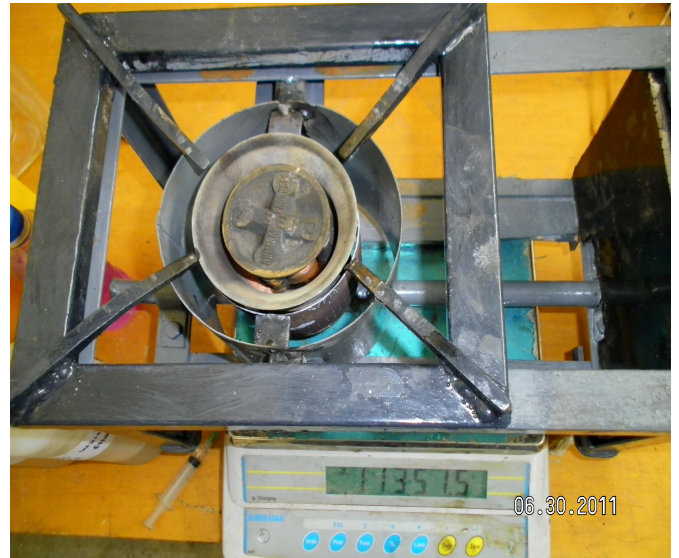
Top view (the stove and weight balance set up)
