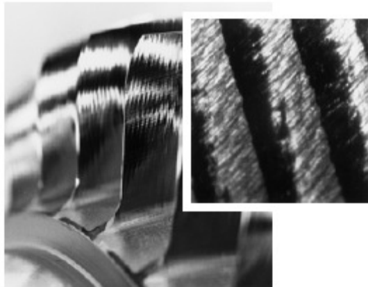
Figure 2.2 Chatter marks on the surface
