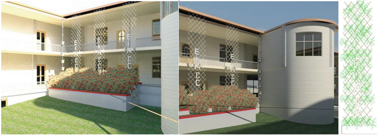
Figure 80: Designed mesh system green façade
