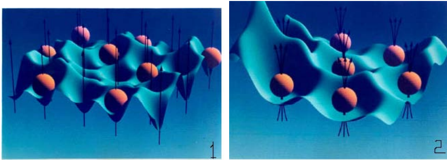
Figure 4.3: The lowest Landau Levels for (1) uncorrelated 1/3 states (2) correlated 1/3 states, wave function of correlated state is \Psi(z_1, z_2, z_3, \dots, z_n) \sim \prod (z_j - z_k)^3 [27].
