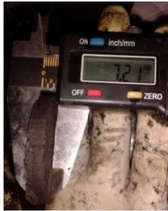
Figure 3-13: Digital clipper used to measure the briquettes thickness
