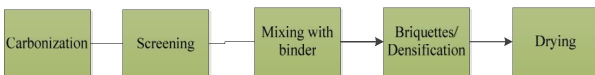
Figure 2-1: Flow diagram for manufacturing Briquettes
