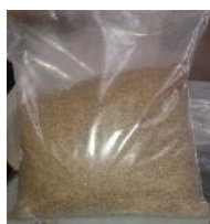
Figure 3-5: The jatropha press cake after the grinding and sieved by < 1mm
