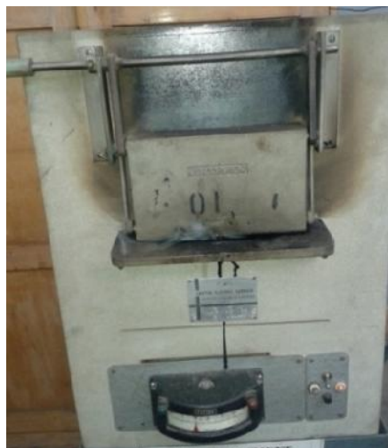
Figure 3-7: Muffle furnace used for carbonized raw material
