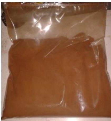
Figure 3-9: Red soils used as a binder
