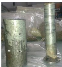
Figure 3-8: Mould used for making briquettes manufacturing in laboratory
