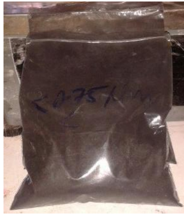
Figure 3-6: Carbonized AR powder after grinding and sieved < 0.75\mu\text{m}
