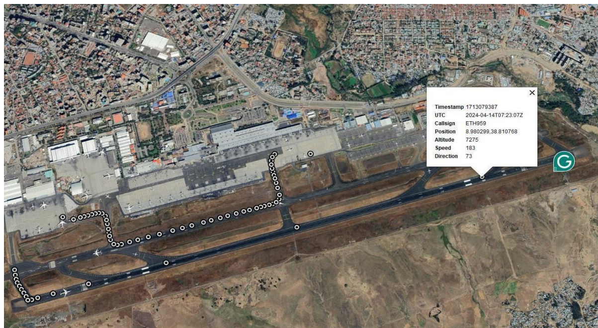
Figure 9 Flight track record sample for an airplane departing from AABIA converted from CSV data using Google Earth
