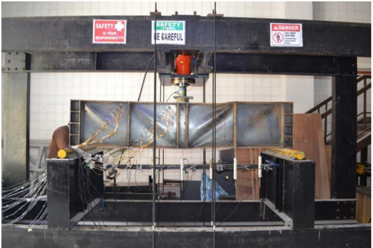
Figure 4-2 Typical test setup and Diagonal buckling formation in typical web panels (Yatim, Azmi and Mukhlisin, 2020)
