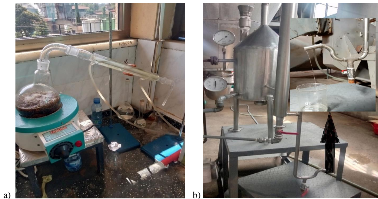
Figure 3.3. Extraction of flavor with (a) Glass in heat mantle and (b) Pot still using steam
