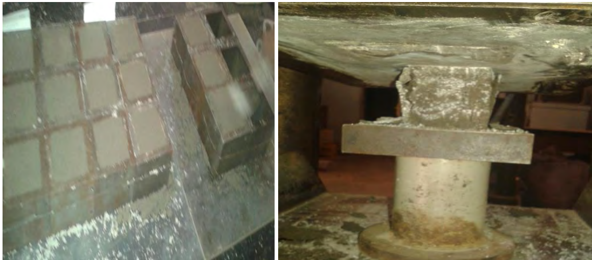
Figure 4-10 Mortar Cube samples (Left) and Compression Test (Right)
