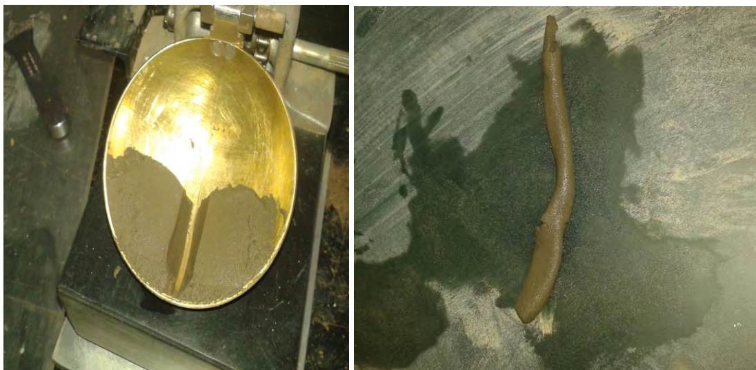
Figure 4-12 Liquid and Plastic limit of Volcanic Ash/Pumicite
