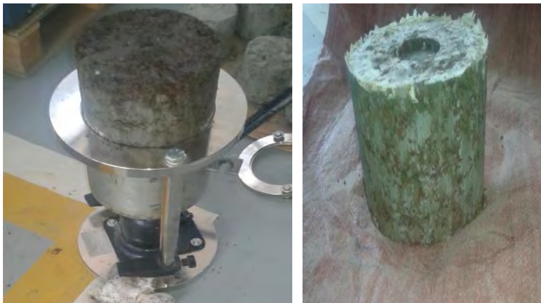
Figure 4-9 Cured and penetrated CBR Sample during Extraction (Left) and after Extraction (Right)
