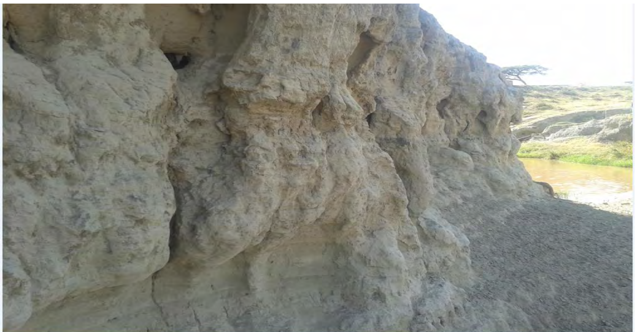
Figure 3-4 Material Site for the Volcanic Ash/Pumicite, picture taken from Ziway Area (a)
