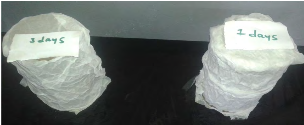
Figure 4-11 three and seven days Cured UCS samples of Volcanic Ash/ Pumicite
