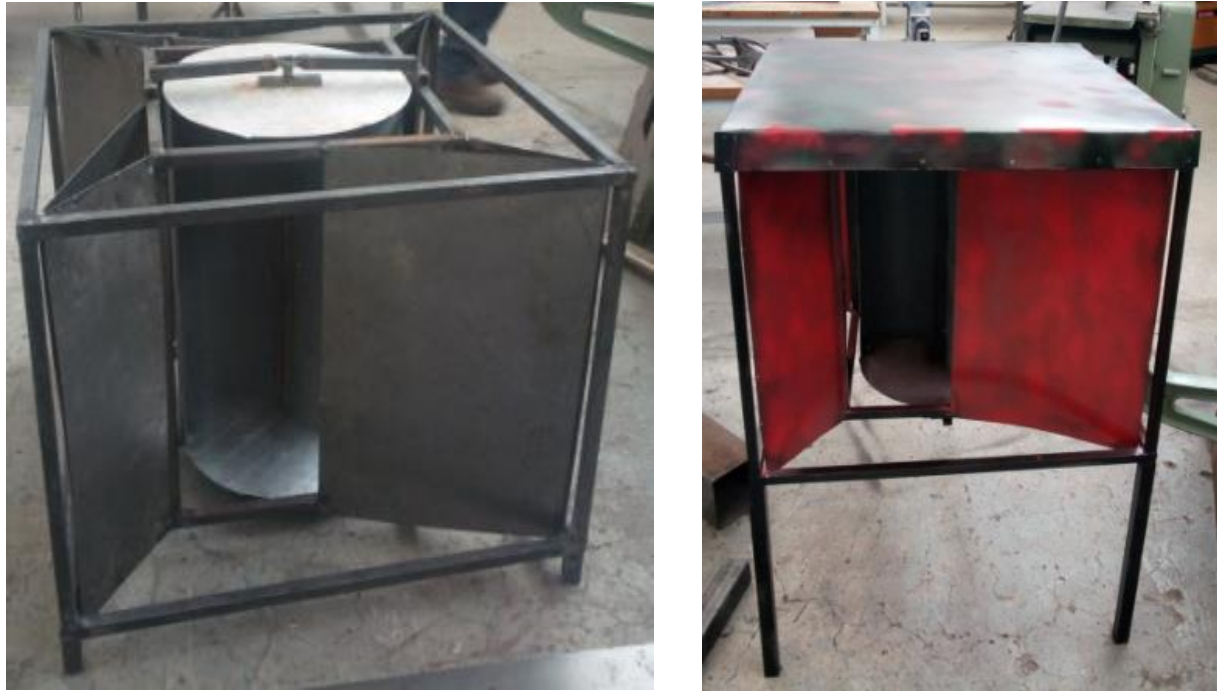
Figure 3. 10: Manufactured model of Savonius wind turbine with air jet mechanism
