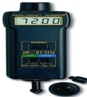
Figure 3. 12: Photo/contact tachometer, DT-2236 [from device manual]
