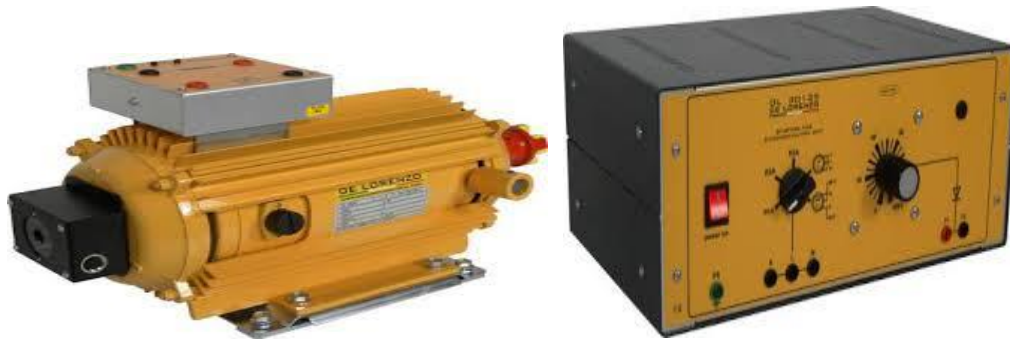
Figure 3. 11: Torque measuring devices [Photo taken in Lab]
