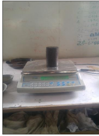
(c) Trimming of sample from the extruded Shelby tube sampler, Measuring the Mass of the specimen and Curing of Sample Specimen for UCS Test
