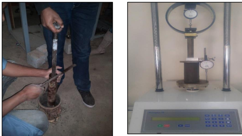
Figure 20: UCS specimen preparation and strength measurement for the native black
