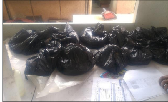
(a) Curing of Sample Specimen for Atterberg Limits Test
