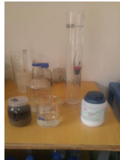
Figure 11: Wet Sieve and Hydrometer tests for the Native Black Cotton Soil
