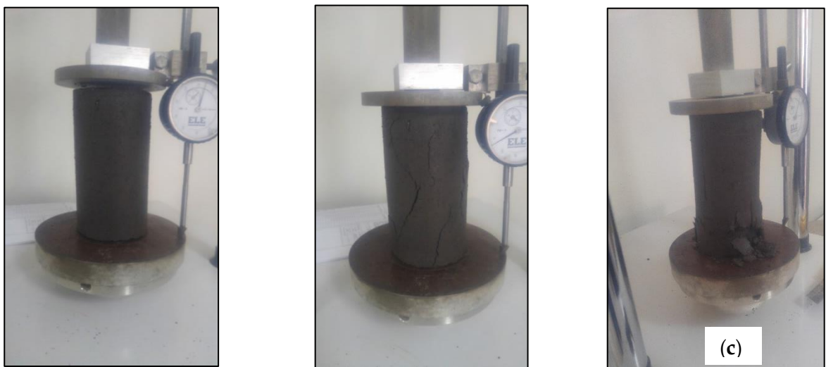
Figure 44: (a) Specimen before compression, (b) Failure mode for the Untreated-soil specimen after UCS test, (c) Failure mode for the soil treated with Cement after UCS test
