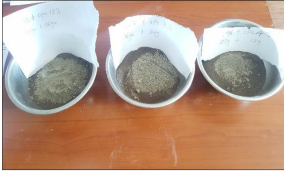
(a) Curing of Sample Specimen for Atterberg Limits Test
