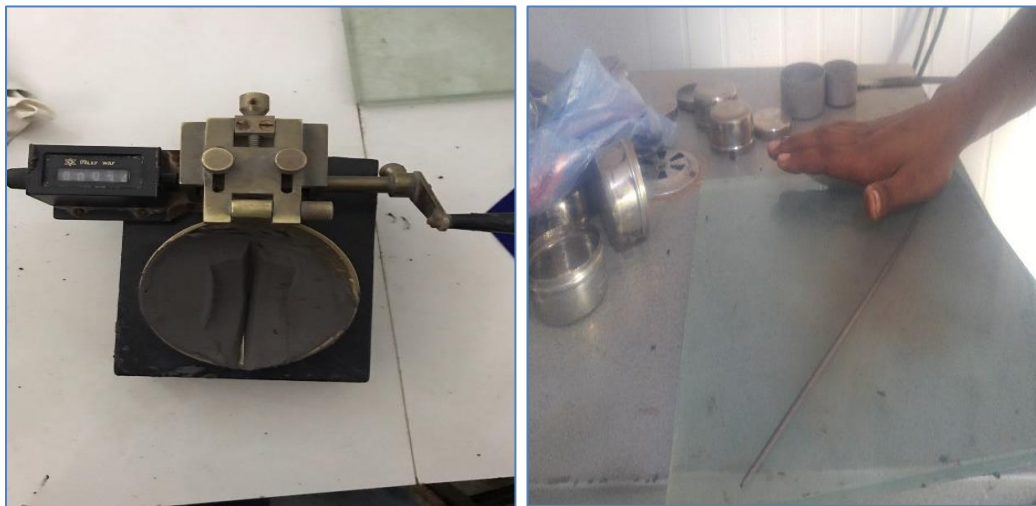
Figure 14: Atterberg Limit tests for the native Black Cotton Soil (Liquid Limit and Plastic Limit tests)
