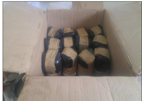
(c) Trimming of sample from the extruded Shelby tube sampler, Measuring the Mass of the specimen and Curing of Sample Specimen for UCS Test
