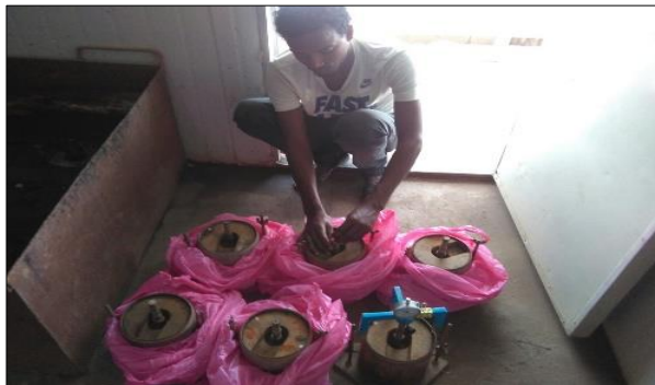
(b) Curing of Sample Specimen for CBR Test
