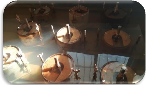
(b) Cement-QD stabilized specimen (annular surcharge discs inside the CBR mold)
