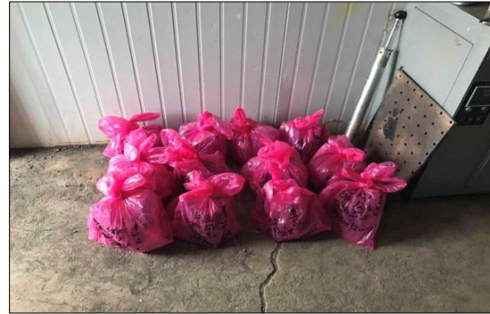
(b) Curing of Sample Specimen for CBR Test
