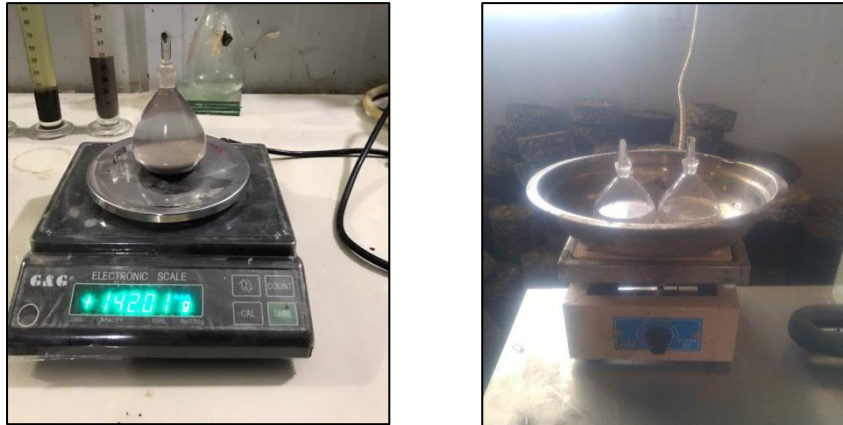
Figure 13: Specific Gravity test for the native Black Cotton Soil
