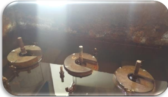
(a) Native Soil (annular surcharge discs outside the CBR mold)
