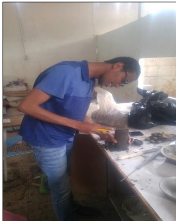
(c) Trimming of sample from the extruded Shelby tube sampler, Measuring the Mass of the specimen and Curing of Sample Specimen for UCS Test
