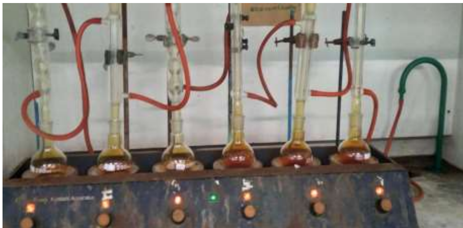
Figure 3. Digesting of soil samples
