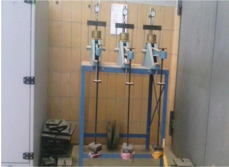
Fig.3.1 One dimensional consolidation test apparatus(AAiT Geotechnical laboratory).
