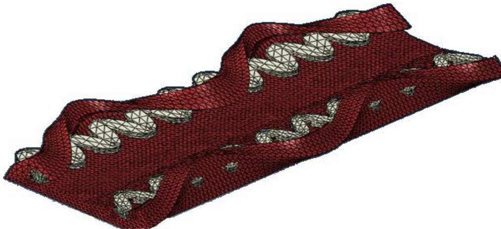
Figure 4-13: 3D BBES Slab and Rail vibration modes in ABAQUS Simulation at frequency 1697Hz
