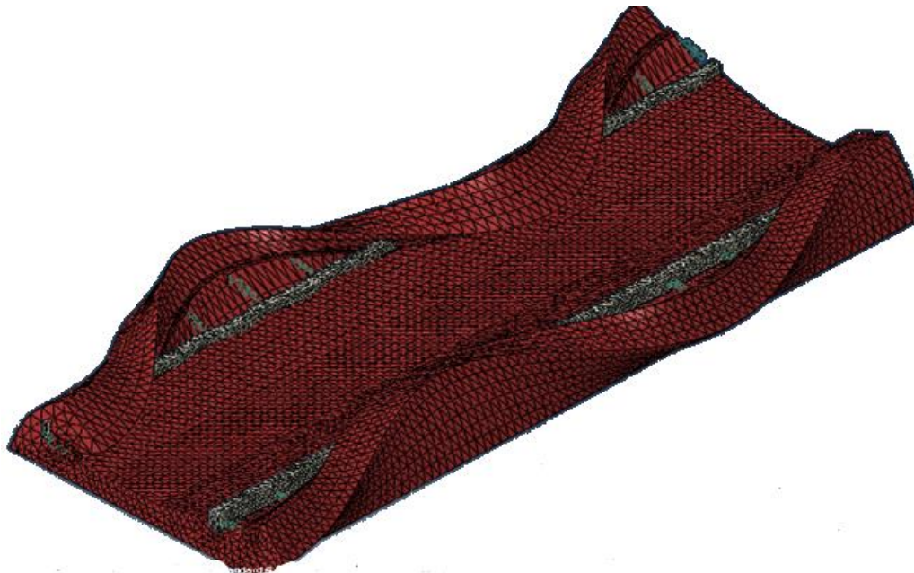
Figure 4-12: 3D BBES Slab vibration modes in ABAQUS Simulation at frequency 1660Hz
