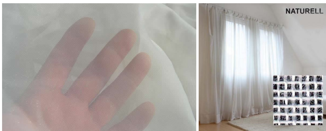
Figure 6: Swiss shield fabric for shielding EMF radiation (source: www.radiansa.com , September 16, 2020)
