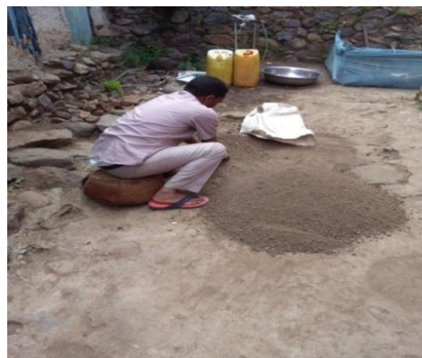
Figure 4: A large composite soil samples were prepared by drying arenosols in sun, powdering this thoroughly so as to ensure sample homogeneity.
