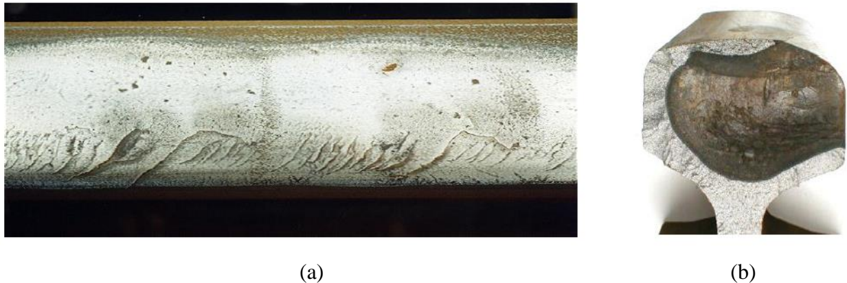
Figure 2.4: (a) Severe Head Checks and (b) cross section of a severe single Head Check [12].
