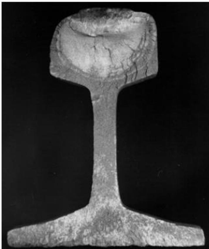
Figure 1.9: “Kidney-shaped” crack in a rail head [4].
