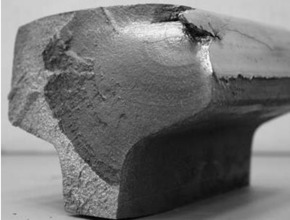
Figure 1.7: Fracture of a rail with origin from a head check [4].
