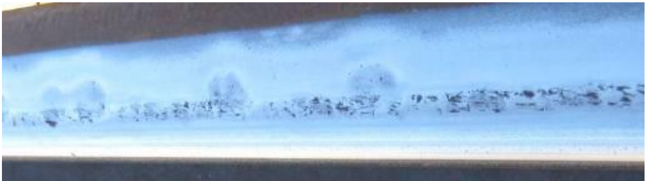
Figure 1.8: Squat: damage of the running surface [4].
