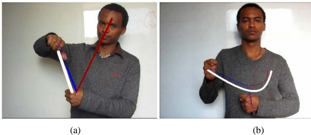
Fig 4.4 Hand Trajectory detection (a) Incorrect detection (b) Correct detection
