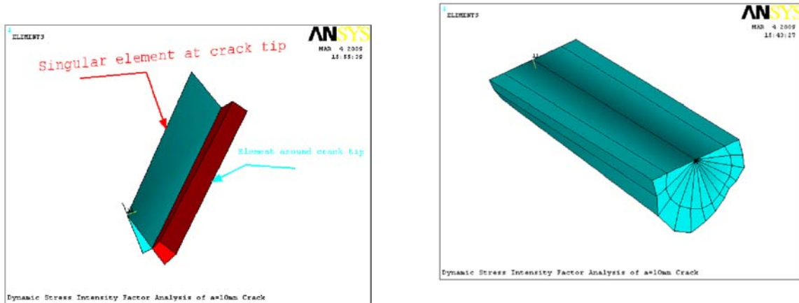
Figure 4.5b longitudinal dimensions of the symmetrical meshed model and half crack length for 20mm crack.
