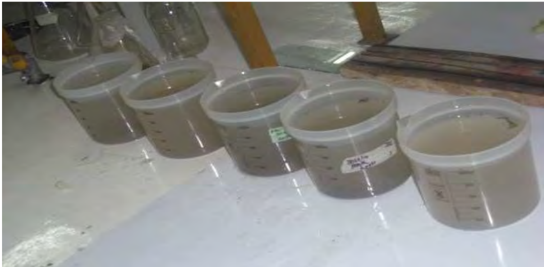
Figure 7: Sedimentation of vegetable washings with physiological saline solution in the laboratory.
