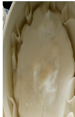
1G. Aged solution 1H. Vacuum filtration of precipitated silica 1I. Filtered silica
