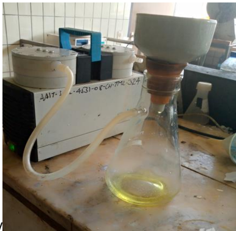
1G. Aged solution 1H. Vacuum filtration of precipitated silica 1I. Filtered silica
