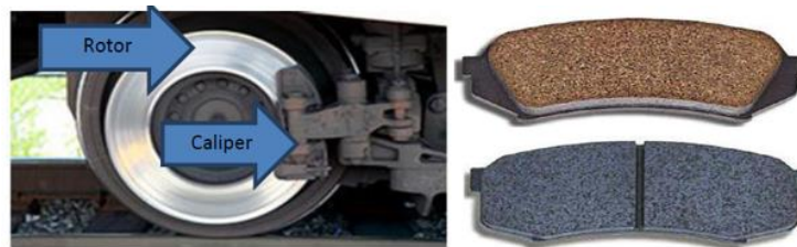
Figure 2.2: Disc brake components[15].
