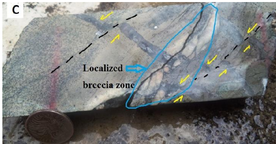
Figure 3.8 small / centimeter scale fault in out crop and core.
