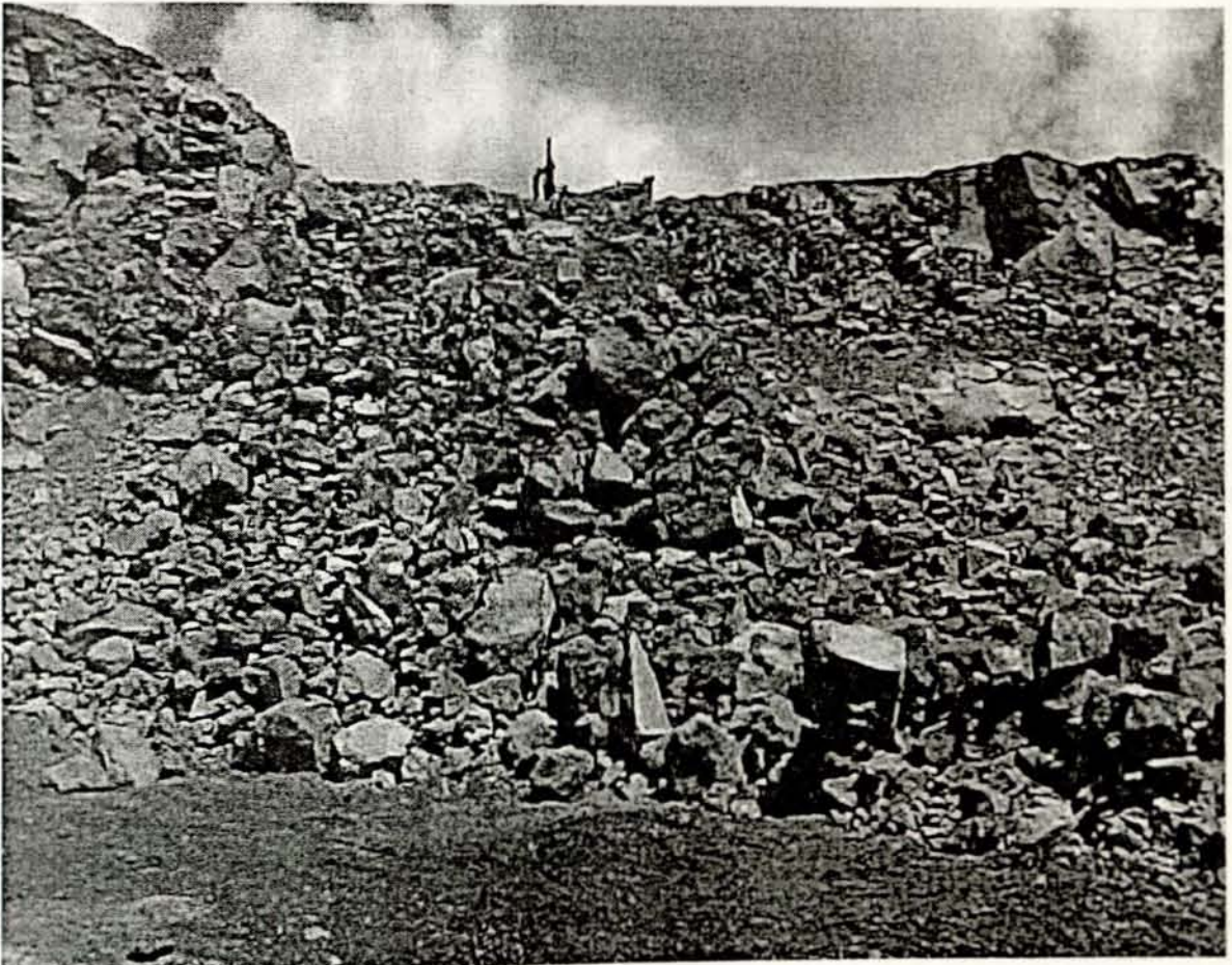
Fig.16. The Fractured Rocks observed After Explosion (at Akaki Quarry)
