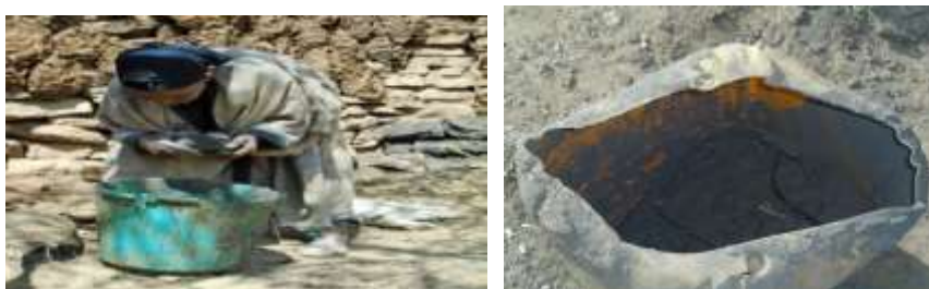
Figure 2. Photo showing a potter immersing clay in water (left) and soaked clay (right)
