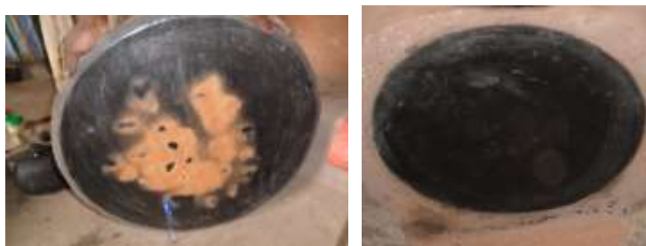
Figure 21. Baking surface of newly fired griddle (left) and griddle in use (right)
