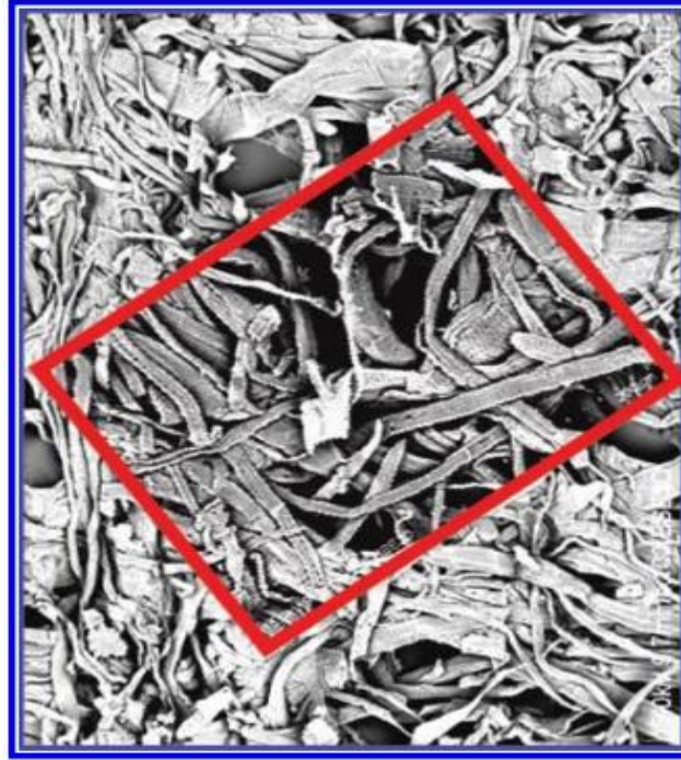
Figure 2.8 Electronic microscopy observation of paper structure (magnification \times 35 and \times 80 in red frame) (Johnston, 2012).
