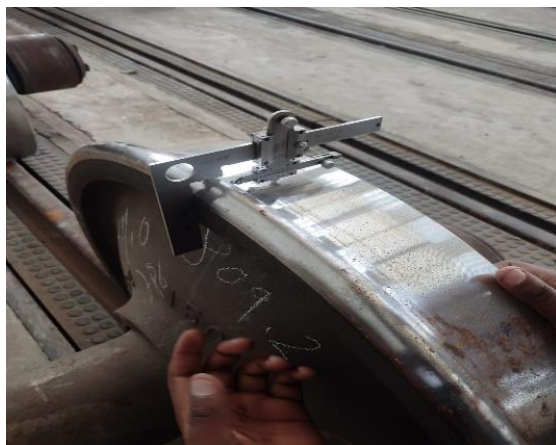
Figure1. 2: Wear on the wheel
