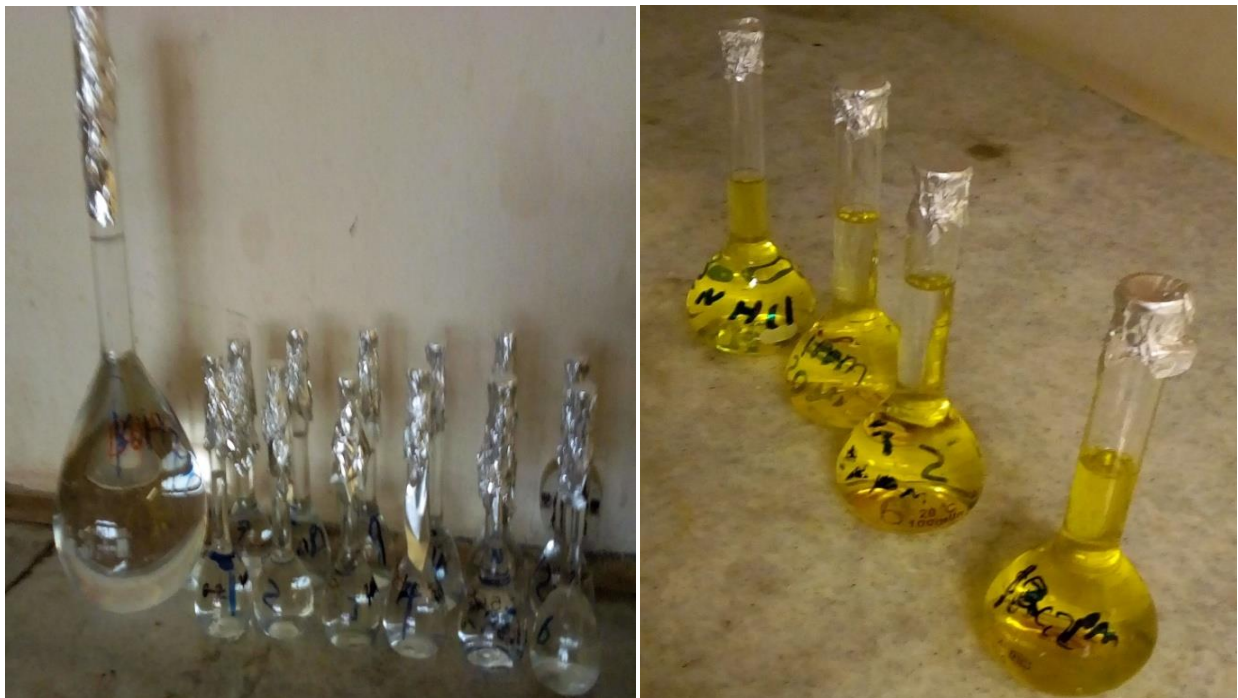
Figure 4: Sample prepared and kept in digestion flask to determine the amount of phosphorus.
