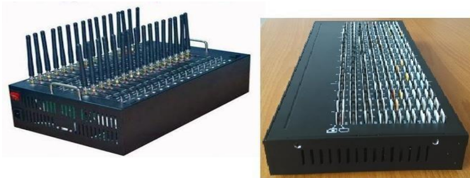
Figure 2.1: Two models of Simbox device (New module 32 SIM card GSM Simbox and 128 SIMs cards call center Simbox device) [1].
