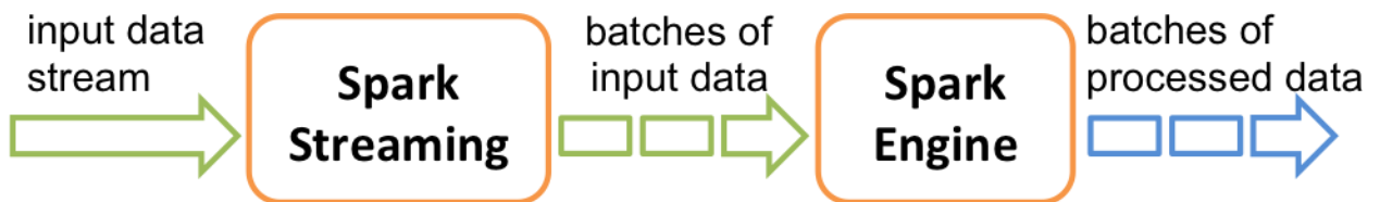
Fig 5.4 Spark Streaming process of creating of Discretized stream [67]
