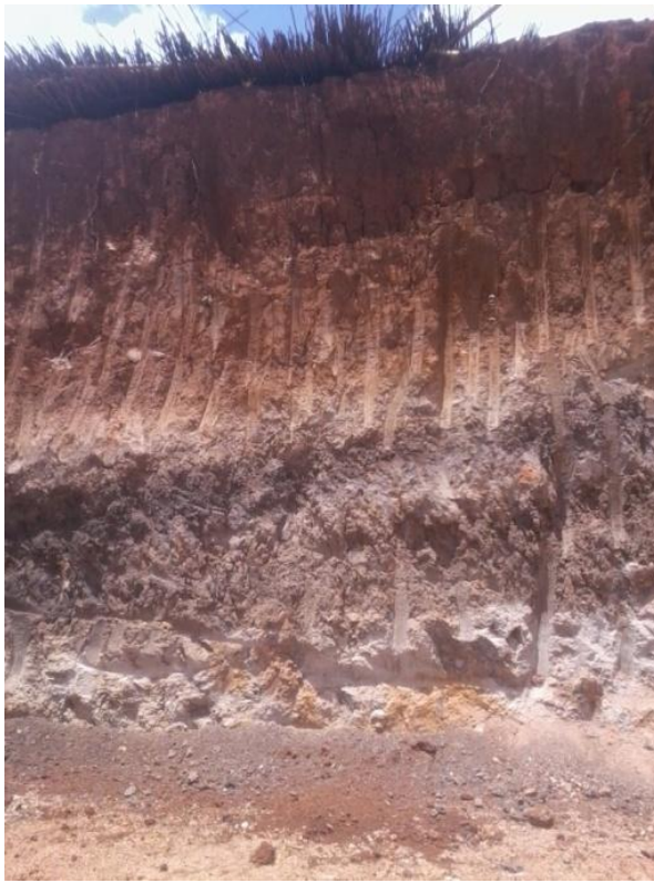
Plate 3.2 a and b- completely weathered rock material
