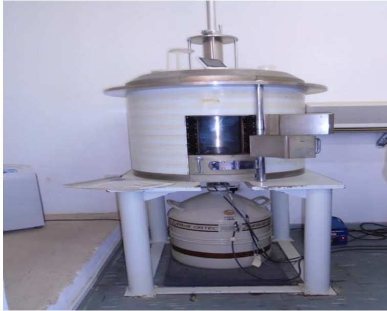
Figure 8: High-purity Germanium HP(Ge) detector inside lead shielding
