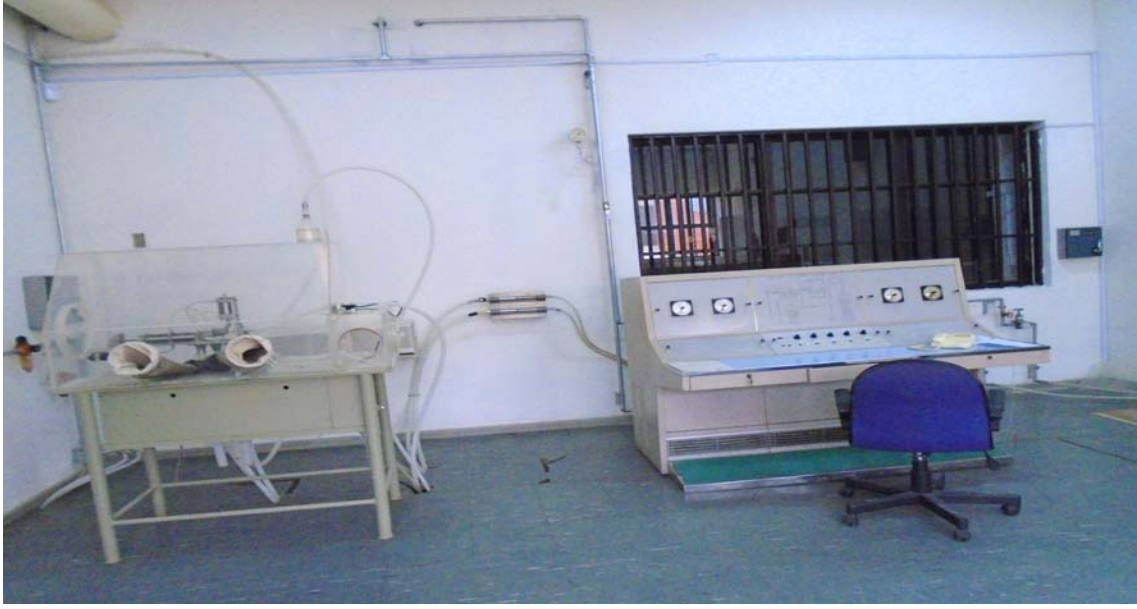
Figure 41: The pneumatic rabbit system of the reactor used during irradiation.
