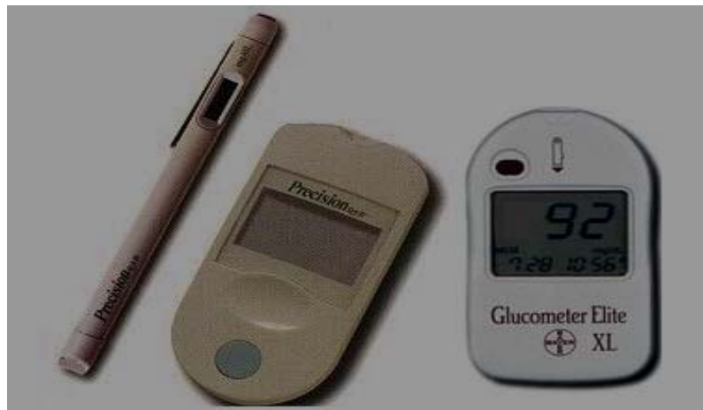
Figure1.1: Images of various types and sizes of the commercially available glucose sensors. The precision glucose test strip (left image) and Glucometers (right image) use the blood samples taken from the Figure tips for measurements [3].
