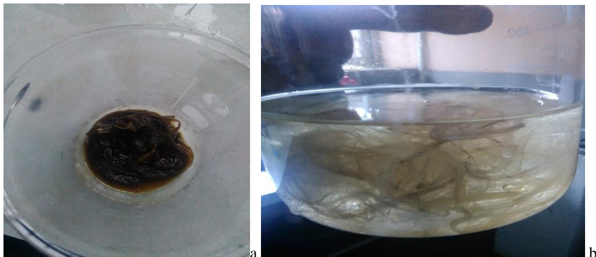
Figure 3-2 mercerization of raw fiber (a fiber with sodium hydroxide solution b) washing with distilled water
