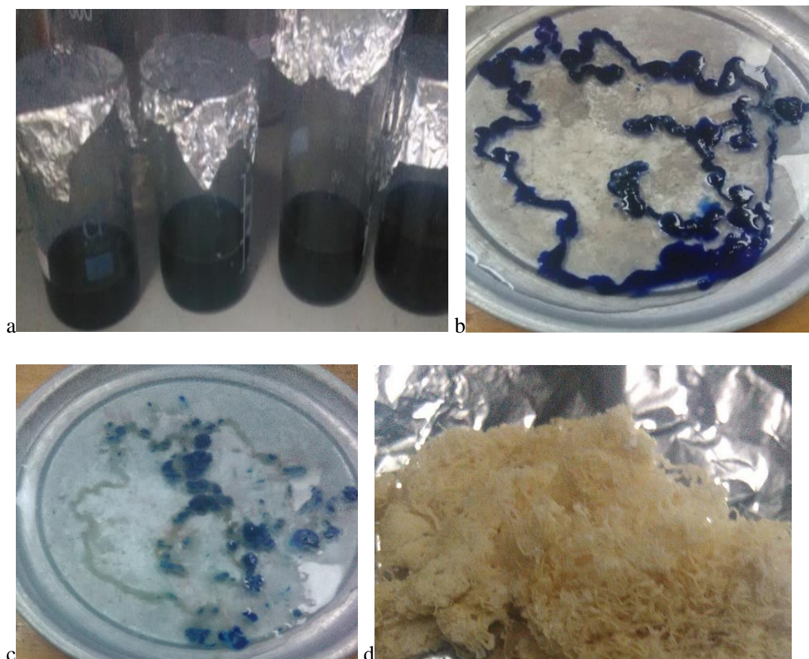
Figure 3-3 process of production of regenerated cellulosic fiber a) reaction of mercerized fiber to copper amine solution, b) injecting to sulfuric acid solution, c) precipitation of regenerated fiber and d) cleaned and put to be dried
