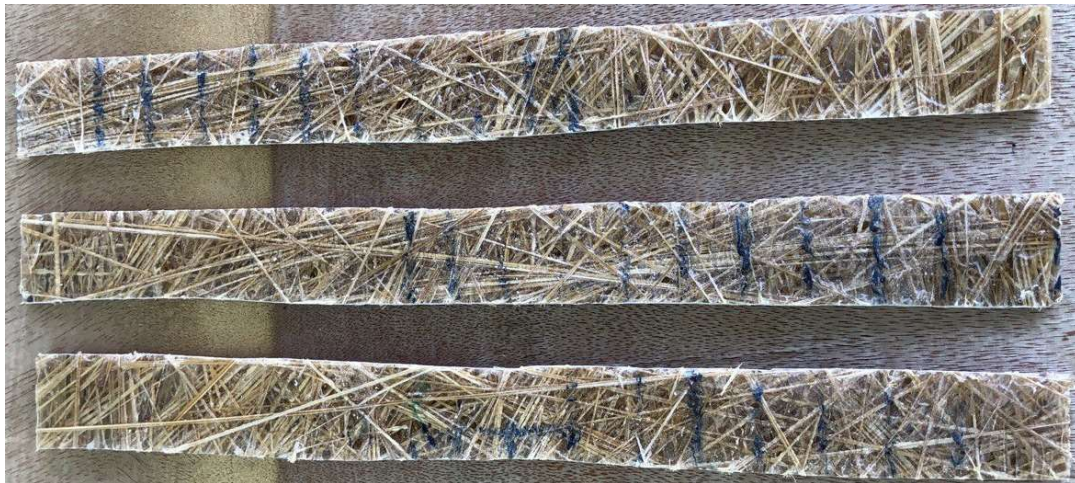
Figure 3.16: Tensile test specimen using woven orientation
