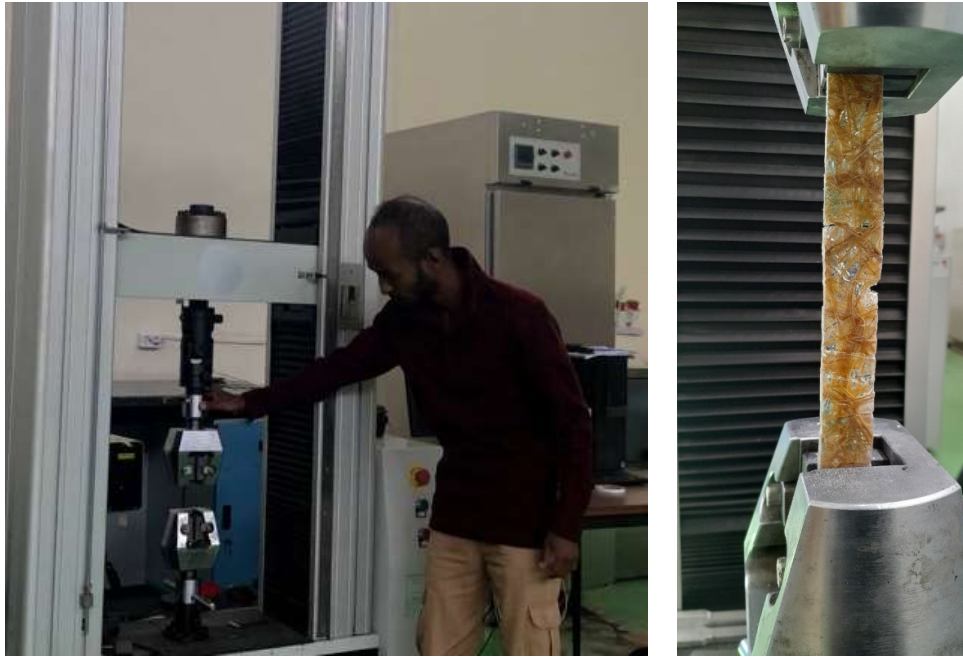
Figure 3.14: Universal Testing Machine (UTM) setup
