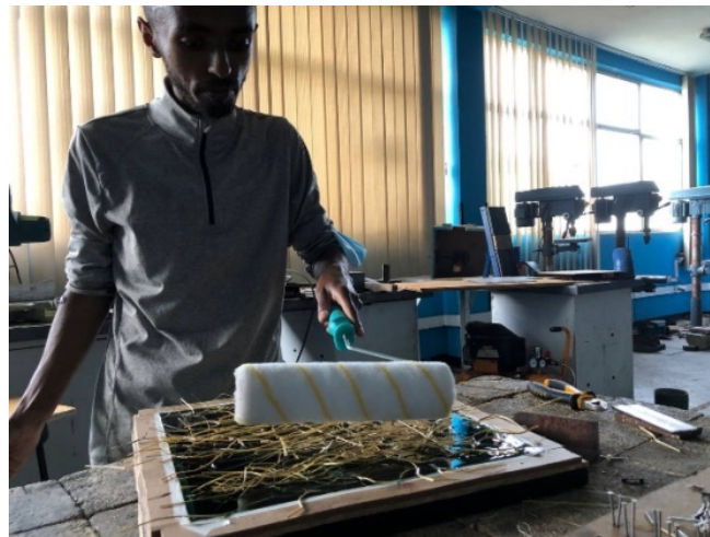
Figure 3.7: Honeycomb-oriented bamboo fiber with epoxy composite preparation
