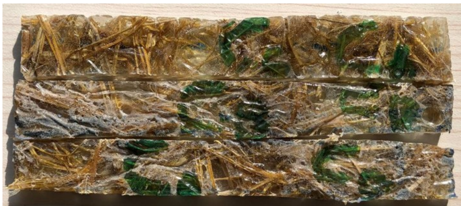
Figure 3.17: Compressive test specimen using honey comb fiber orientation
