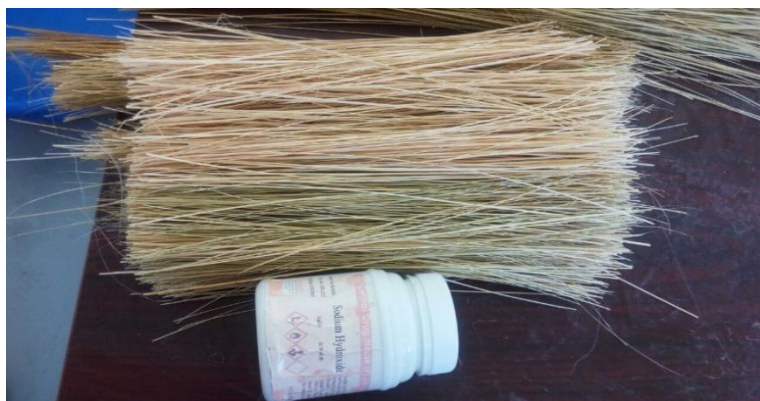
Figure 3.3: Extracted bamboo fibers manually
