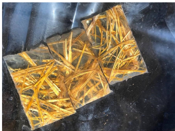
Figure 3.23: Water Absorption Test Specimen using honeycomb orientations
