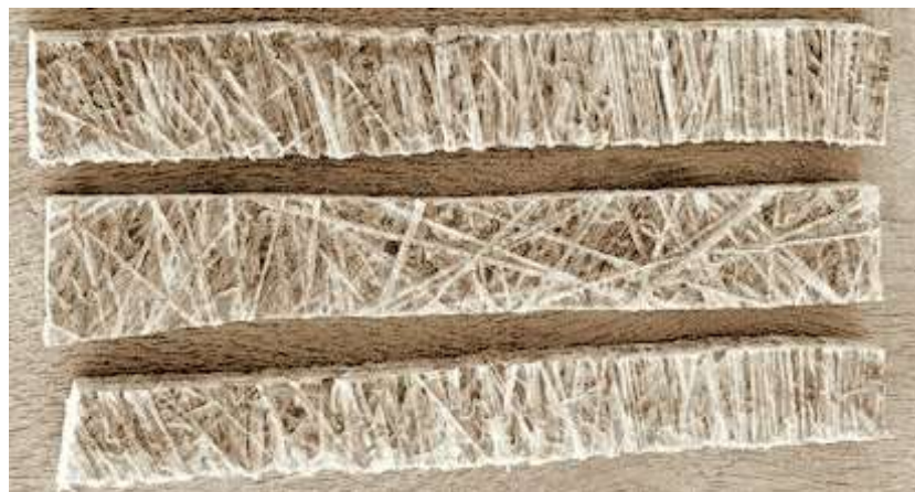
Figure 3.20: Flexural Strength Test Specimen using woven orientation
