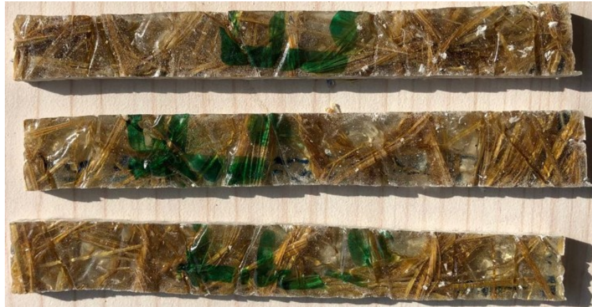
Figure 3.19: Flexural strength test specimen using honey comb orientation
