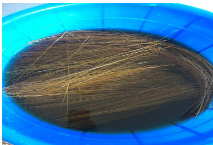
Figure 3.4: Bamboo fiber alkaline treatment
