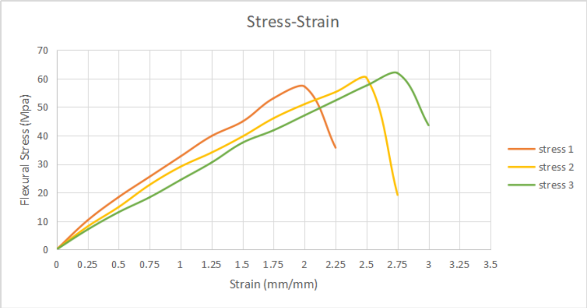
Figure 4.21: Flexural test results of the Bamboo/epoxy composite
