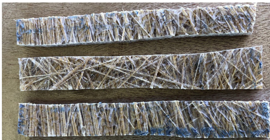
Figure 3.18: Compressive Test Specimen using woven orientation
