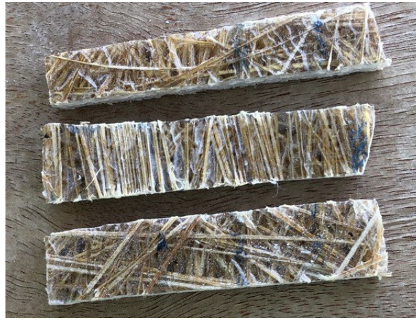
Figure 3.22: Impact Strength Test Specimen using woven orientation
