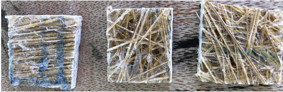
Figure 3.24: Water Absorption Test Specimen using woven orientation
