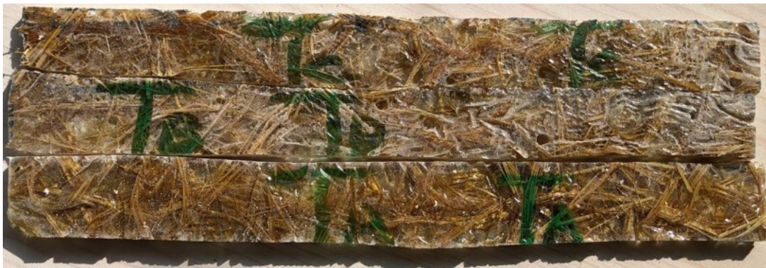
Figure 3.15: Tensile test specimen using honeycomb fiber orientation
