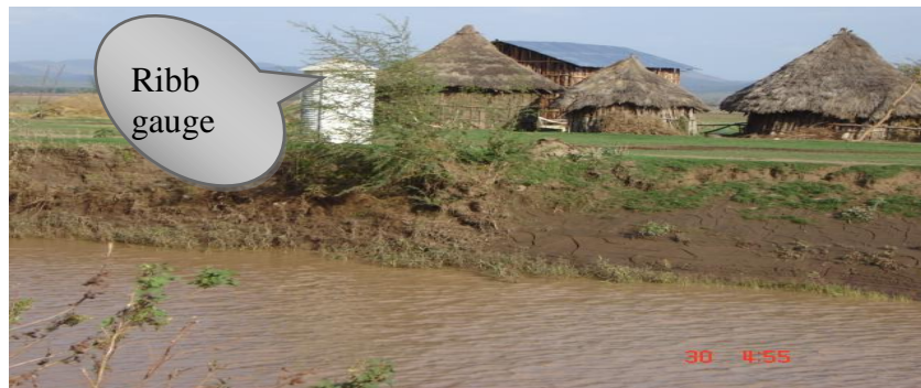
Figure 18: Staff Gauges Fixed at unstable River Bank
