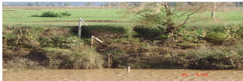
Figure 19: Staff Gauges Fixed at Ribb River Bank
