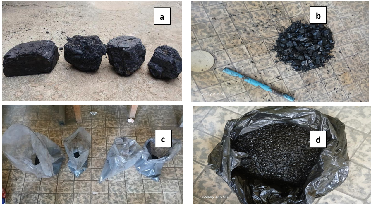
Figure 14 : Comminution (Size Reduction) Process in the Laboratory, showing (a) Raw Coal (b) Crushed Coal (c) Quartering of Coal (d) Grounded Coal
