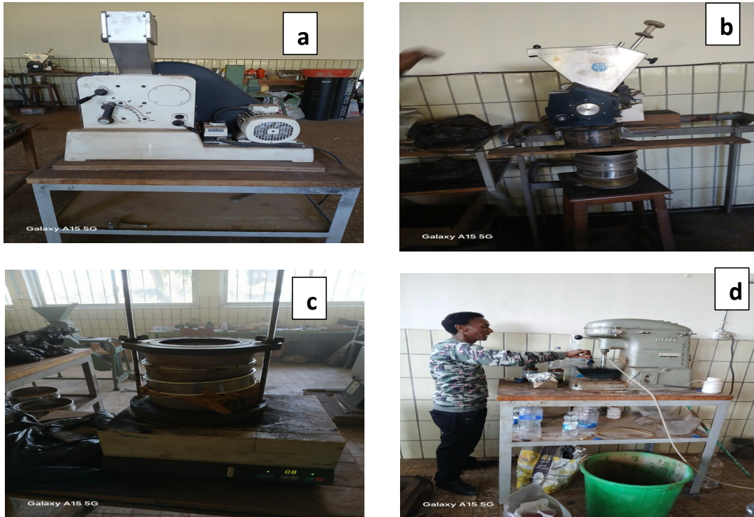
Figure 13 : The lab equipment used in this project (a) Centrifugal Grinder (RETCH 56402 Deutschland) for laboratory purposes; (b) Jaw Crusher for laboratory use (RoHs53743) (c) Various mesh-sized sieves & Sieve Vibrator (RETCH A200, Deutschland) (d) Flotation Unit (Wedag Groppe 98, West Deutschland)
