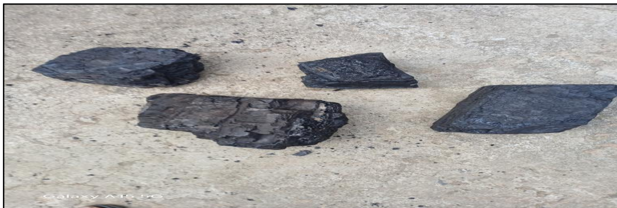
Figure 10: Tarcha Coal rock sample, very lustrous, highly compacted, high strength and demonstrate sub conchoidal fracture (Mengistie, T. M. 2018).
