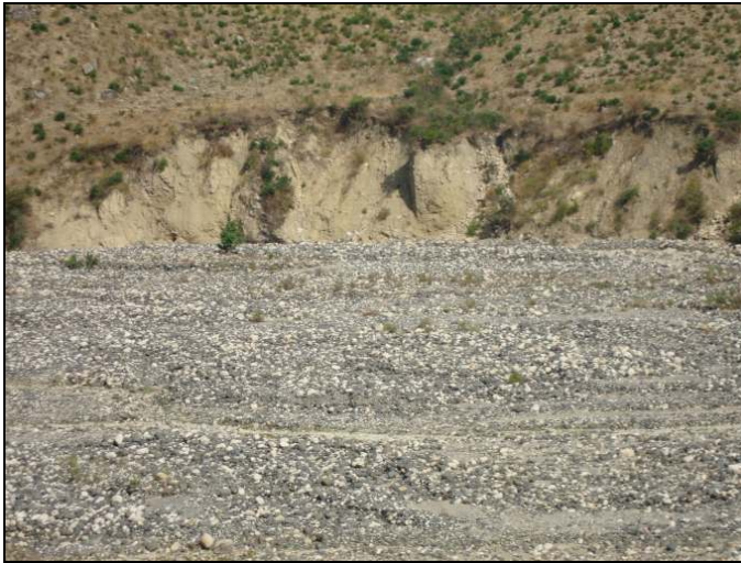
Figure 14: River sand laying on river bed and colluvial material deposited at the river bank
