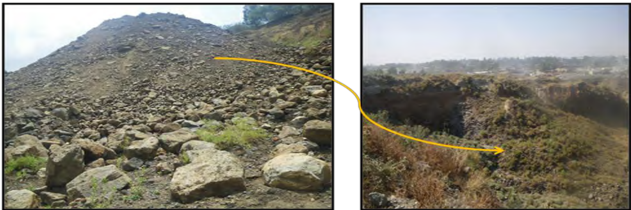
Figure 24: the stripped overburden material from the active mining site used to refilling the abandoned quarry site in the study area
