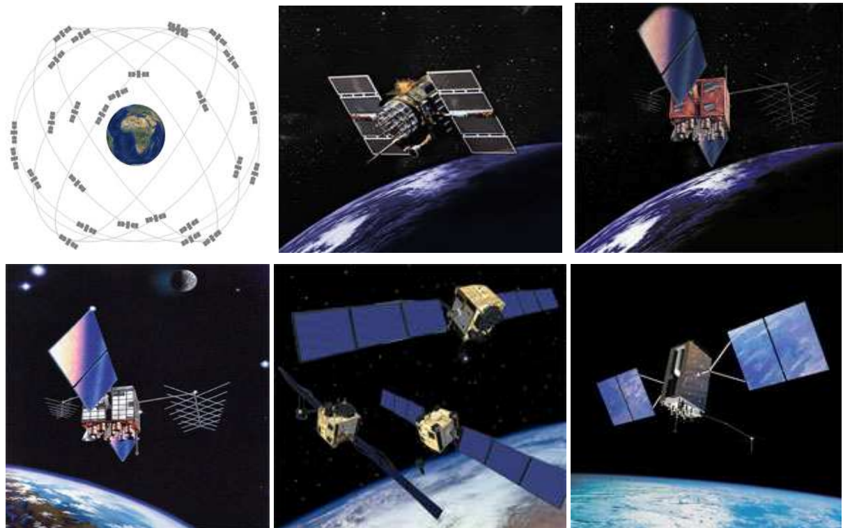
Figure 2. 2: GPS space segment showing GPS satellite constellation (top left), GPS Block IIA (top middle), GPS Block IIR (top right), GPS Block IIR-M (bottom left), GPS Block IIF (bottom middle), and GPS Block III satellite (bottom right). (Source: http://www.gps.gov/systems/gps/space/ ).
