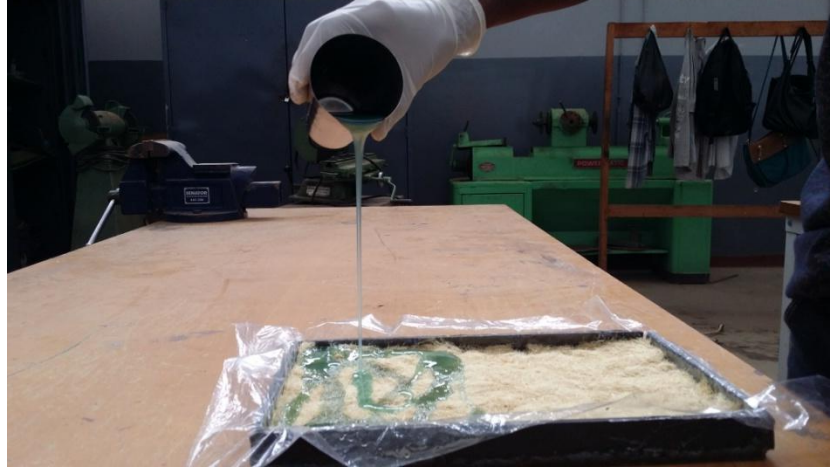
Figure 3-11 Sisal fiber reinforced epoxy composite molding at AAIT Lab
