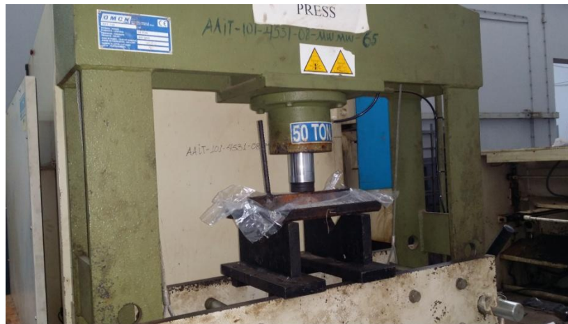
Figure 3-12 Standard Hydraulic Press for curing
