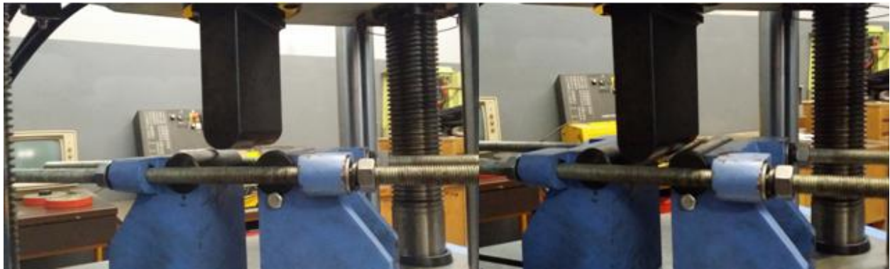
Figure 3-19 Specimen under flexural testing
