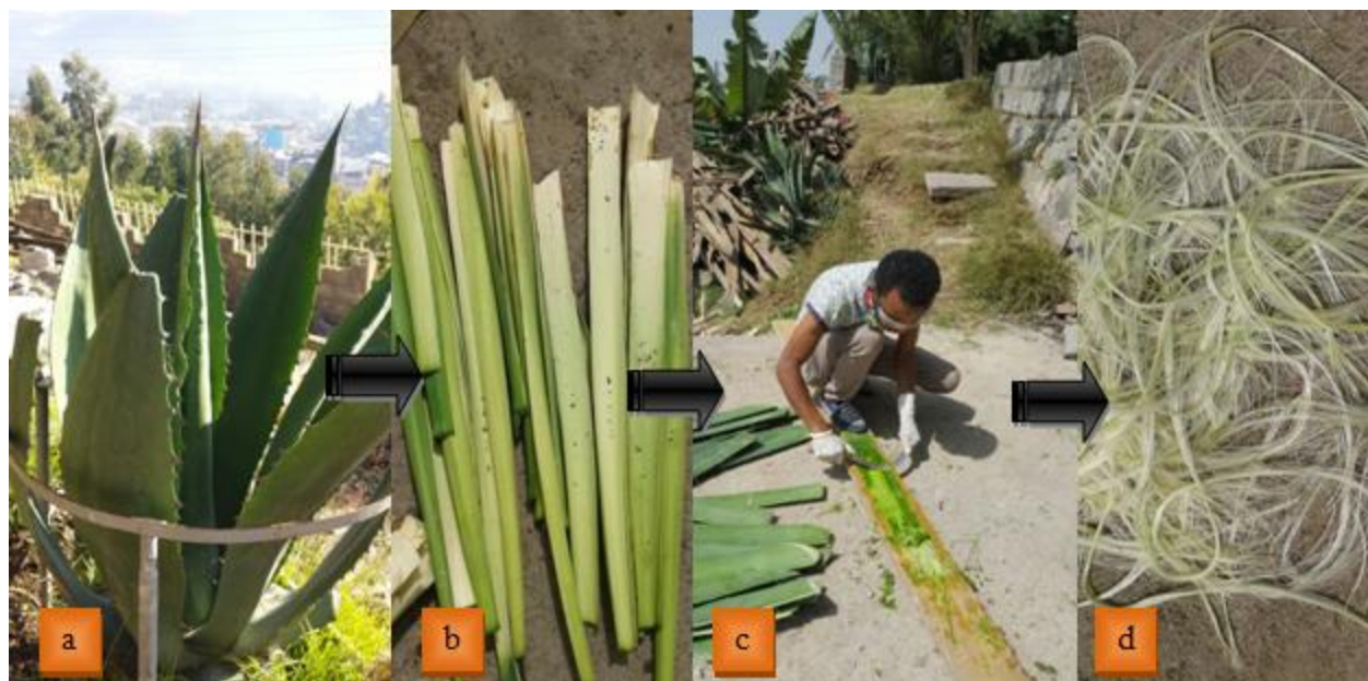
Figure 3-1: Sisal fiber extraction process a, Sisal plant b, longitudinally trimmed sisal plant c, peeling of sisal plant for sisal fiber extraction d, Extracted sisal fiber before washing and drying
