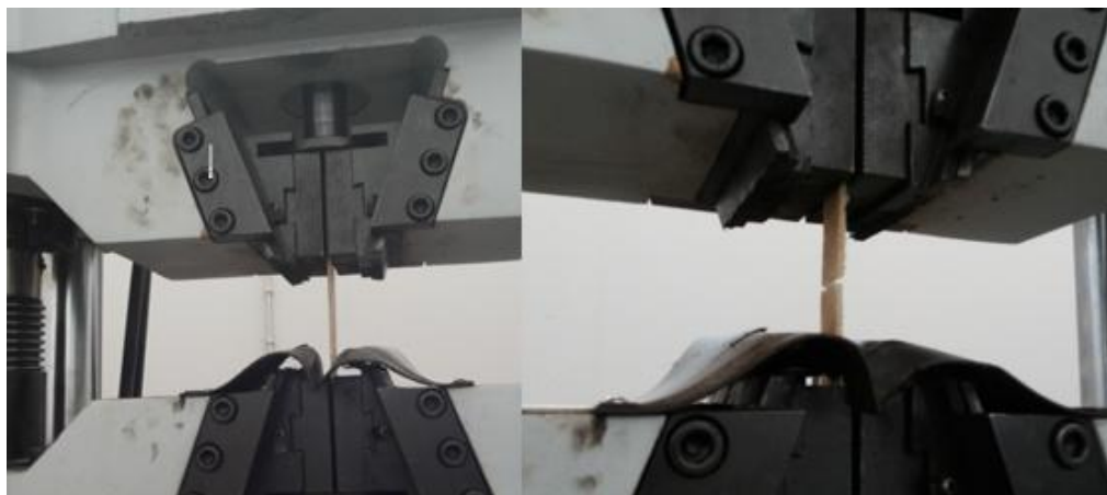
Figure 3-21 Typical specimen under tensile strength test
