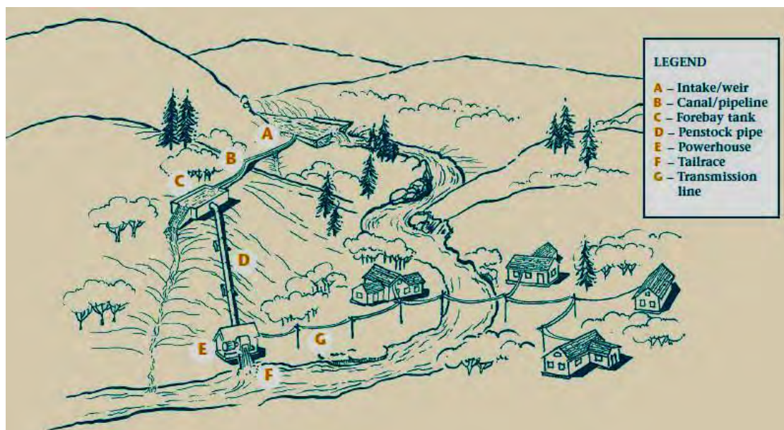
Figure2.1. Typical layout of micro hydropower system [13]
