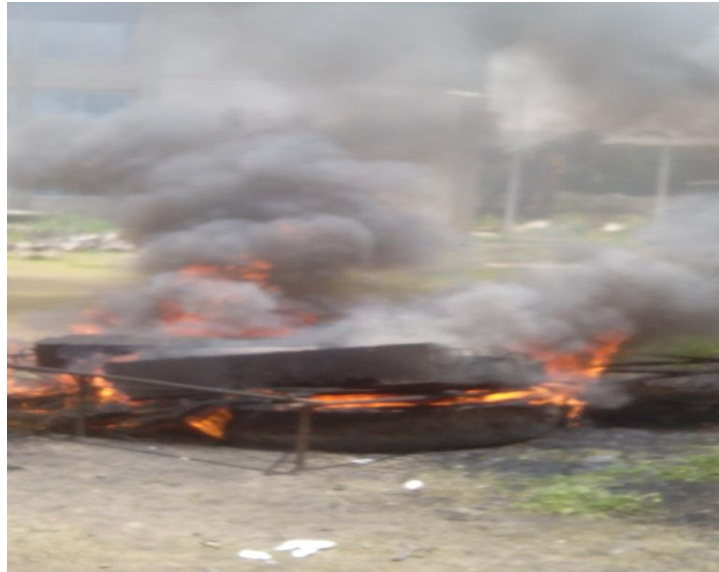
Fig.3.15- sample beam under intensified burning
