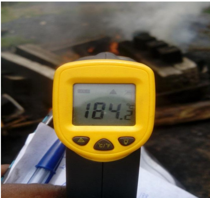
Fig.3.7- Infrared thermometer measuring temperature of concrete surface.
