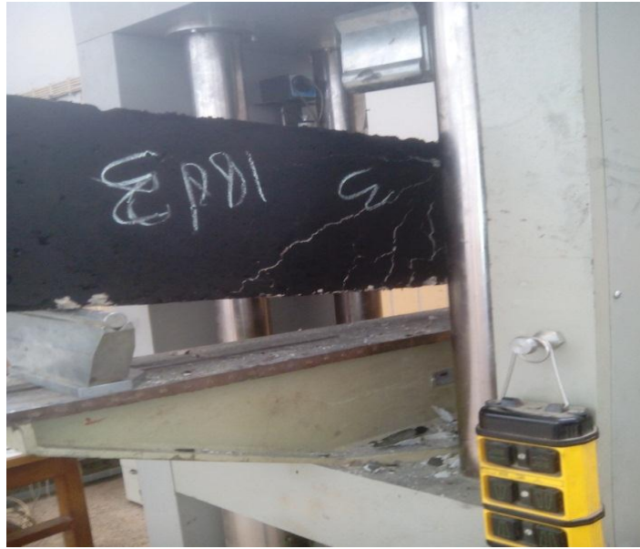
Fig.3.17- Sample beam testing in loading machine after failure.
