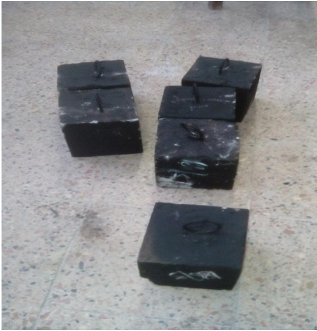
Fig.3.8- Concrete cubes air cooled to room temperature ready for test
