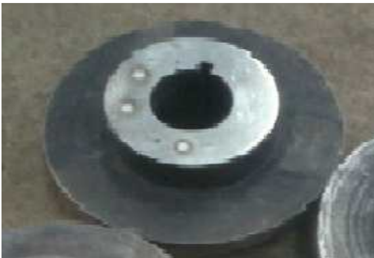
Figure 3.10 burnt test roller after chemical composition test
