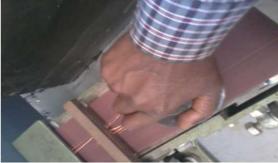
Figure 3.9 Roller preparations on belt sander for chemical composition test
