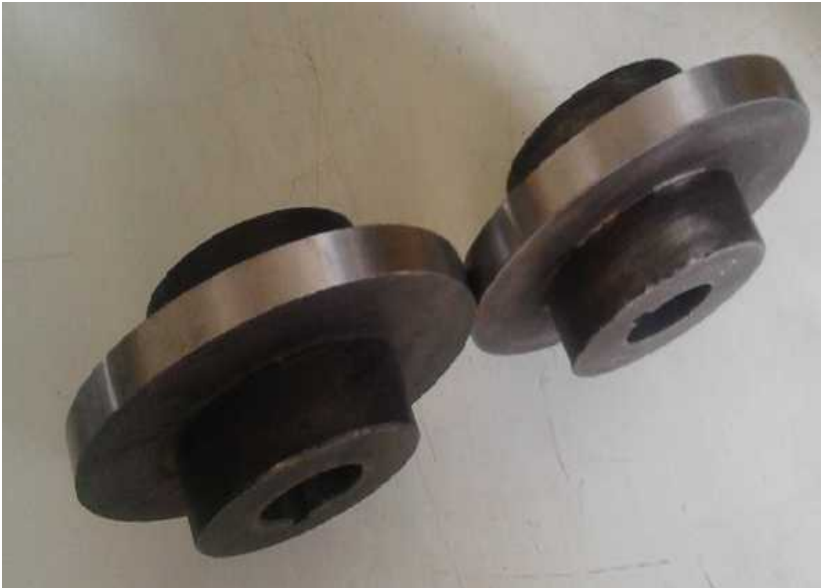
Figure 3.1 Specimen of roller for rolling/sliding wear test [6]
