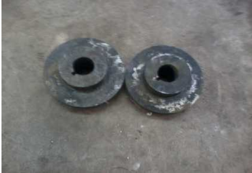
Figure 3.7 pair of rollers quenched in water
