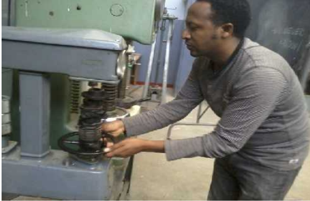
Figure 3.8 Hardness testing on Rockwell C scale of rollers
