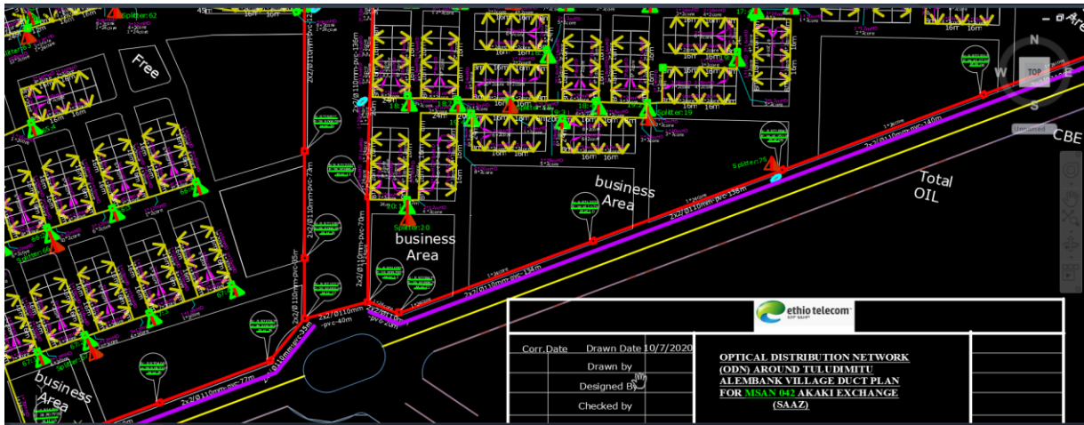
Figure 5. 3 Sample of duct plan for civil works [48].
