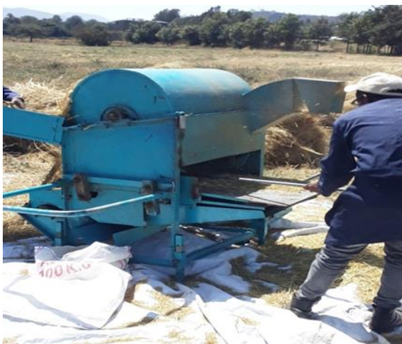
(a) Field performance of teff thresher Test at DEBREZEIT
