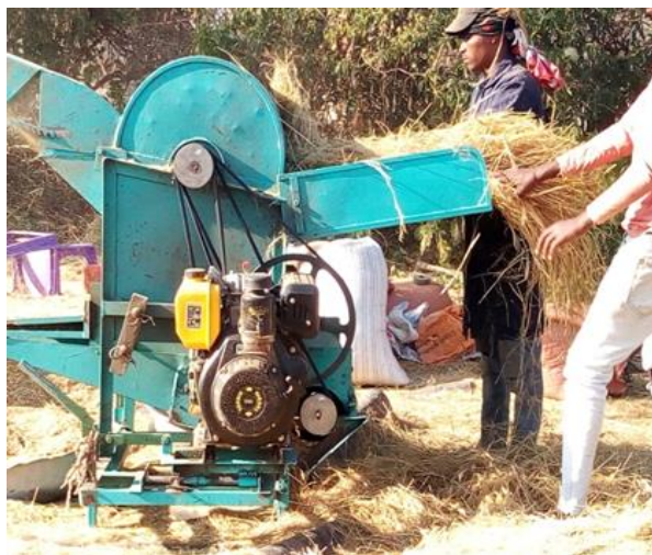
(b) Field performance test of teff thresher awash Melkassa Waketiyo
