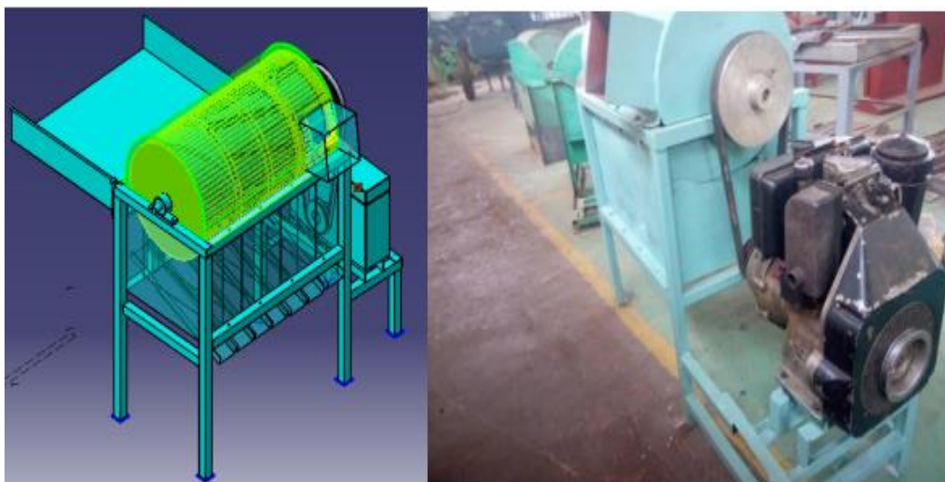
Figure 2-8 Teff thresher developed by Geta Kidanemariam Gelaw [3]
