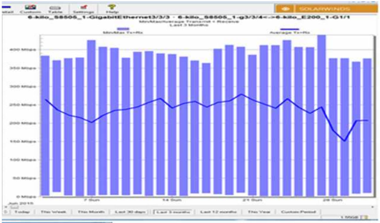
Figure 4.5 Weekly Minimum, maximum and Average data transmitted and received from 6kilo Core switch in June
