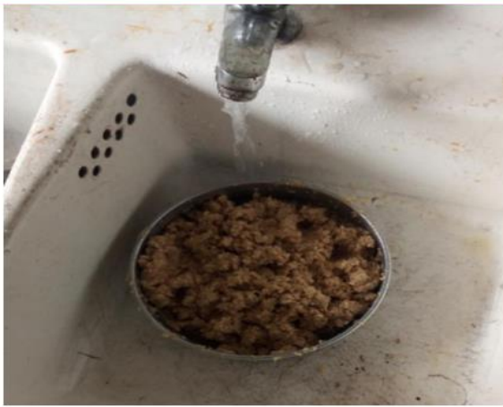
Raw material pretreatment for characterization and production of AC
