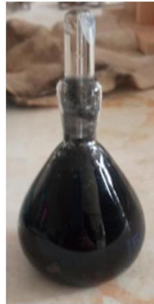
Bulk Density measurement of activated carbon by pycnometer
