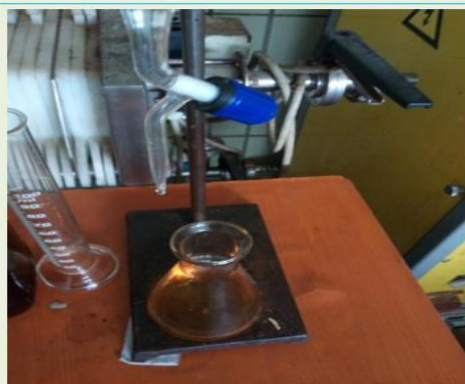
Experimental setup during iodine number determination, AAiT, AAU-research Lab
