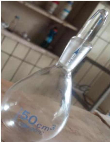
Bulk Density measurement of activated carbon by pycnometer
