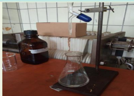
Experimental setup during iodine number determination, AAiT, AAU-research Lab
