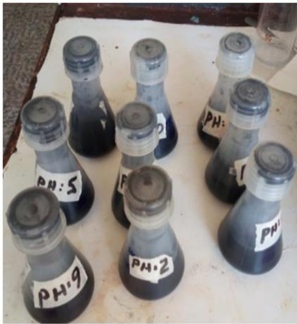
Point of Zero Charge Determination for flax straw activated carbon
