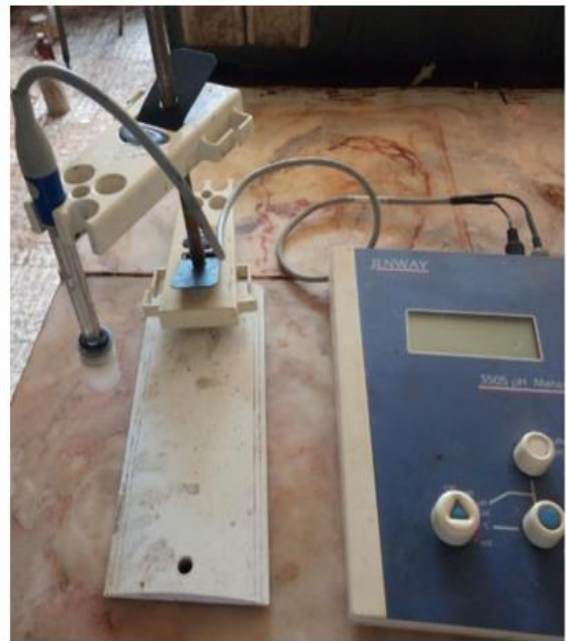
Point of Zero Charge Determination for flax straw activated carbon
