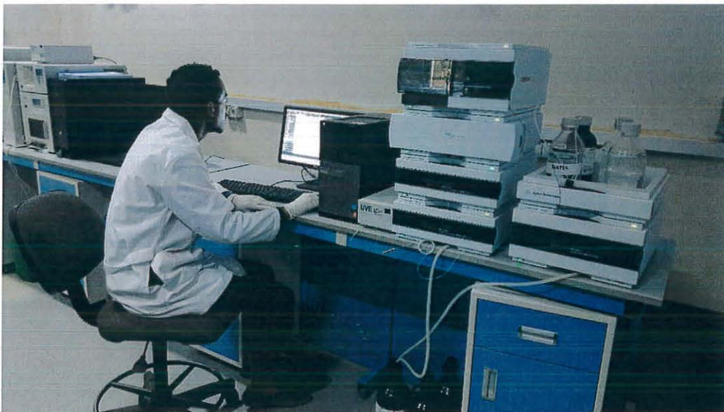
Figure 11. Identification of acrylamide using HPLC-DAD in the laboratory
