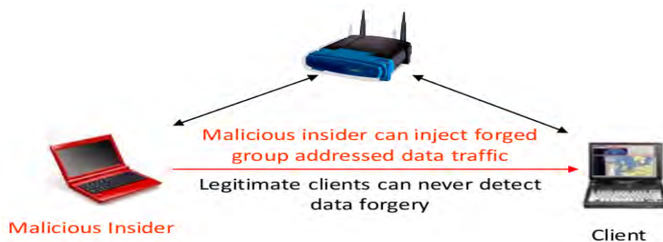
Figure 2.11: Injection of Forged Group Addressed Data Traffic
