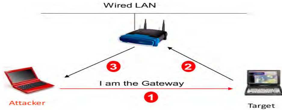
Figure 2.12: ARP Poisoning in Wireless LAN
